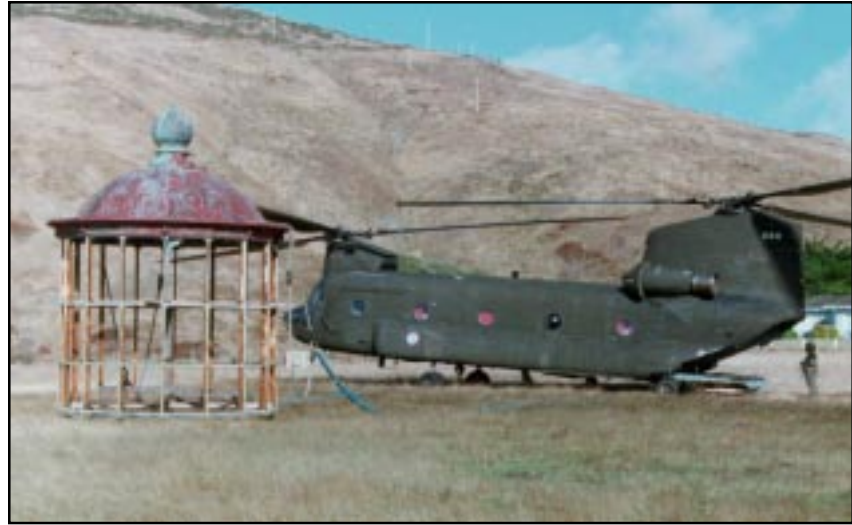
Mission Completed! The dome of the historic Cape Mendicino Lighthouse perches in Mel Coombs Park after a slingload ride under a “Delta Schooners” Chinook from its old resting place on Cape Mendicino. □
