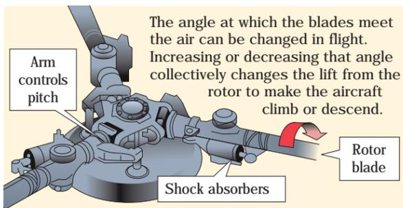
The angle at which the blades meet the air can be changed in flight. Increasing or decreasing that angle collectively changes the lift from the rotor to make the aircraft climb or descend.
