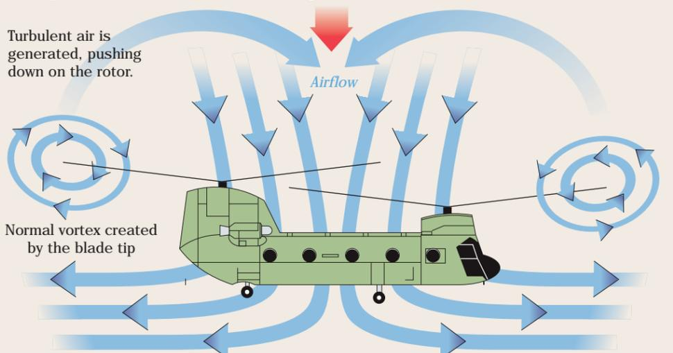
The full power of the engines is not enough to overcome the sink rate, resulting in a crash.
