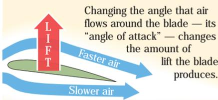
Changing the angle that air flows around the blade — its "angle of attack" — changes the amount of lift the blade produces.
