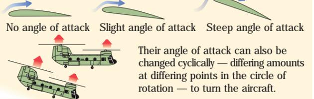
Their angle of attack can also be changed cyclically — differing amounts at differing points in the circle of rotation — to turn the aircraft.
