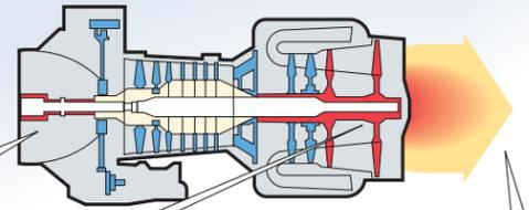
Air enters through the engine intake and is ducted to the compressor section.
