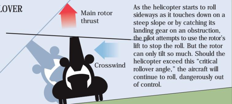
As the helicopter starts to roll sideways as it touches down on a steep slope or by catching its landing gear on an obstruction, the pilot attempts to use the rotor's lift to stop the roll. But the rotor can only tilt so much. Should the helicopter exceed this "critical rollover angle," the aircraft will continue to roll, dangerously out of control.
